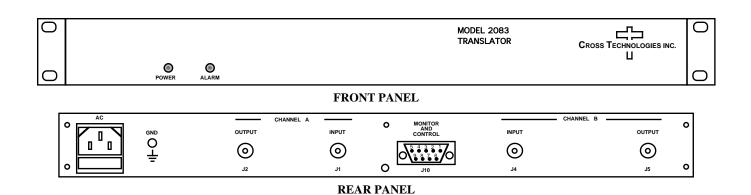
FIGURE 1.1 Front and Rear Panels
