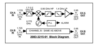
FIGURE 1.2 Block Diagram
