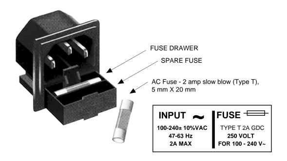
FIGURE 2.3 Fuse Location and Spare Fuse
